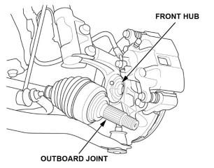
15. Wipe off any grease contamination from the tapered ball joint section and threads, then install the knuckle onto the lower arm. Make sure not to damage the ball joint boot.
