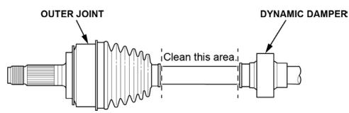
3. Using a ruler and yellow paint marker, measure **40 mm (1-11/16 in)** away from the dynamic damper, and mark the driveshaft with a dot. Click <u>HERE</u> to view a video on how to do the inspection procedure.
