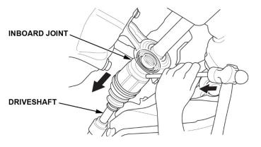
10. Driver's side driveshaft only: Replace the set ring on the inboard joint.
