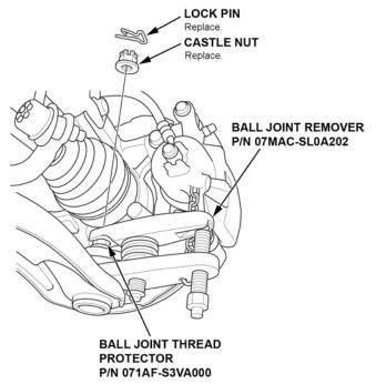
4. Separate the ball joint from the knuckle using the Ball Joint Thread Protector (T/N: 07AAF-SDAA100) and Ball Joint Remover (T/N: 07MAC-SL0A202). Grease the threads and tip of the pressure bolt on the ball joint remover, and make sure the pivot bolt is not parallel to the ball joint remover arms. For additional information on how to use the tools, refer to the service information.
