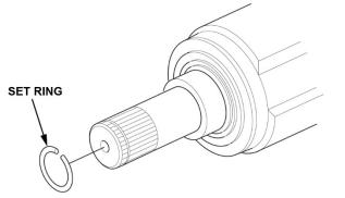
11. Passenger's side driveshaft only: Replace the set ring on the intermediate shaft.
