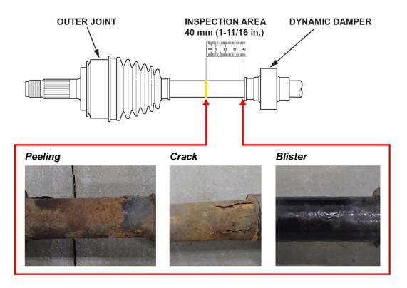
Is there peeling paint, cracks, or blisters on either driveshaft within 40 mm (1-11/16 in) of the dynamic damper?
