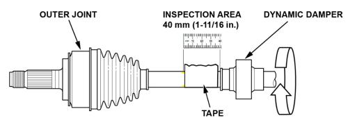
6. Using the masking tape as a guide, trace a line all around the axle using the yellow paint marker. Marking the line accurately is important, especially if there is damage close to or inside the 40 mm line.
