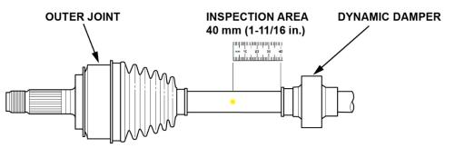
4. Rotate the axle 1/4 turn and repeat the step above **three times** until there are four paint dots on the axle.
