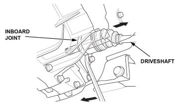
9. *Passenger's side driveshaft only*: Using a punch and hammer, drive the inboard joint off of the intermediate shaft. Then, remove the driveshaft as an assembly.
