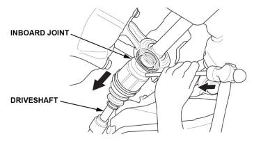
10. Driver's side driveshaft only: Replace the set ring on the inboard joint.
