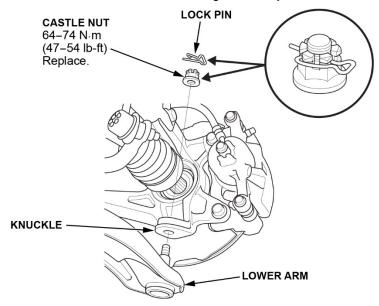
17. Install the new castle nut, and torque it to the lower torque specification. Then, tighten it until the slot on the castle nut aligns with the ball joint pin hole. Install the lock pin into the pin hole as shown.
