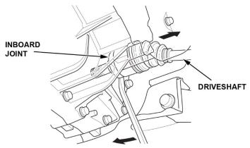
9. *Passenger's side driveshaft only*: Using a punch and hammer, drive the inboard joint off of the intermediate shaft. Then, remove the driveshaft as an assembly.
