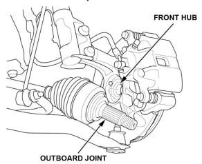
16. Wipe off any grease contamination from the tapered ball joint section and threads, then install the knuckle onto the lower arm. Make sure not to damage the ball joint boot.
