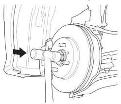
6. Pull the knuckle outward to separate the outboard joint from the front wheel hub.
