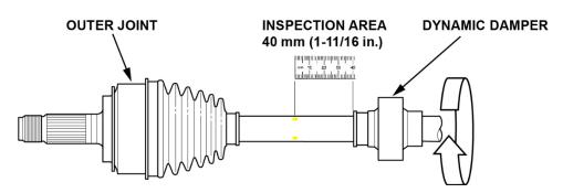
5. Connect the four painted dots around the axle using masking tape.
