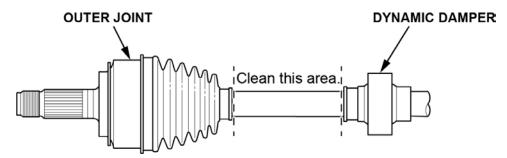
3. Using a ruler and yellow paint marker, measure **40 mm (1-11/16 in)** away from the dynamic damper, and mark the driveshaft with a dot. Click HERE to view a video on how to do the inspection procedure.
