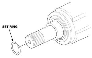
11. Passenger's side driveshaft only: Replace the set ring on the intermediate shaft.
