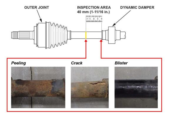
Is there peeling paint, cracks, or blisters on either driveshaft within 40 mm (1-11/16 in) of the dynamic damper?
