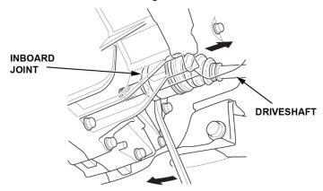
8. *Passenger's side driveshaft only*: Using a punch and hammer, drive the inboard joint off of the intermediate shaft. Then, remove the driveshaft as an assembly.
