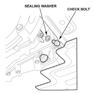
The transmission is at the proper level if the fluid is dripping from the hole gradually.
