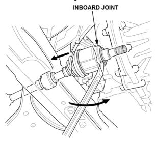
6. Remove the left driveshaft as an assembly.
