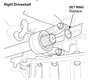
10. Install the new driveshafts. Insert them until the set rings lock in the grooves.
