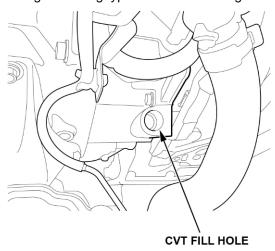
23. Install the filler cap in the direction shown and restart the procedure at step 17.
