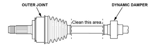
3. Using a ruler and yellow paint marker, measure **40 mm (1-11/16 in)** away from the dynamic damper, and mark the driveshaft with a dot. Click <u>HERE</u> to view the video on how to do the inspection procedure.
