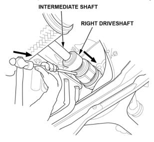
8. Remove the right driveshaft as an assembly.
