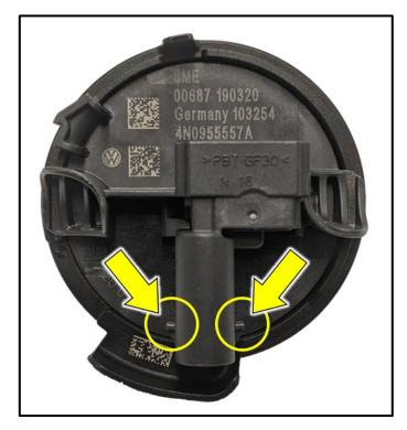
Inspect left and right Front Passenger Thorax Airbag Crash Sensors -G179/G180- and replace if necessary.
