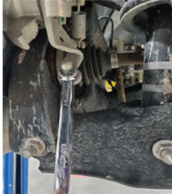
**(3) Replace the Caliper Body Assembly**
