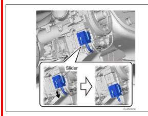
(i) Slide the slider to release the lock, and then disconnect the airbag connector
