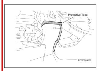
(i) TIP: apply protective tape to the position indicated in the illustration to prevent damage to the LOWER NO. 2 INSTRUMENT FINISH PANEL.
