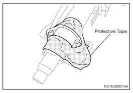
Cover the areas other than the steering actuator bolts with protective tape, so that the steering lock actuator assembly, which is to be reused, is protected from metal debris.
