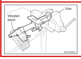
Use a vice to secure the steering column assembly for extracting the interlock bolts.
