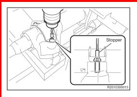
Hold the drill straight and make a hole 10mm deep
