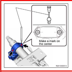
Mark the center of the two interlock bolts with a spring-loaded center punch.
