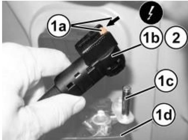
**Figure 19 – Battery Negative Cable**
