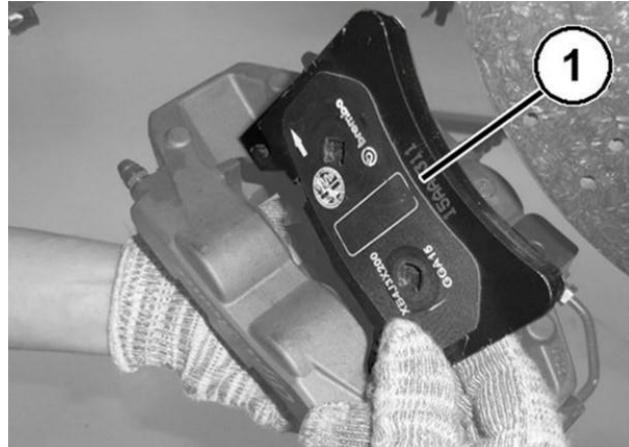
**Figure 8 – Outer Brake Pad**
