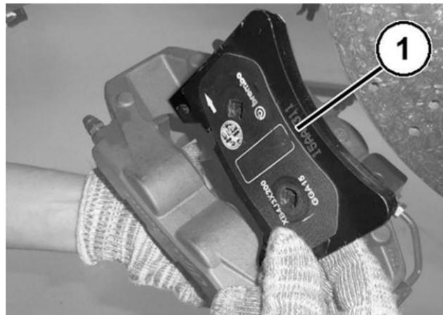
**Figure 15 – Outer Brake Pad**
