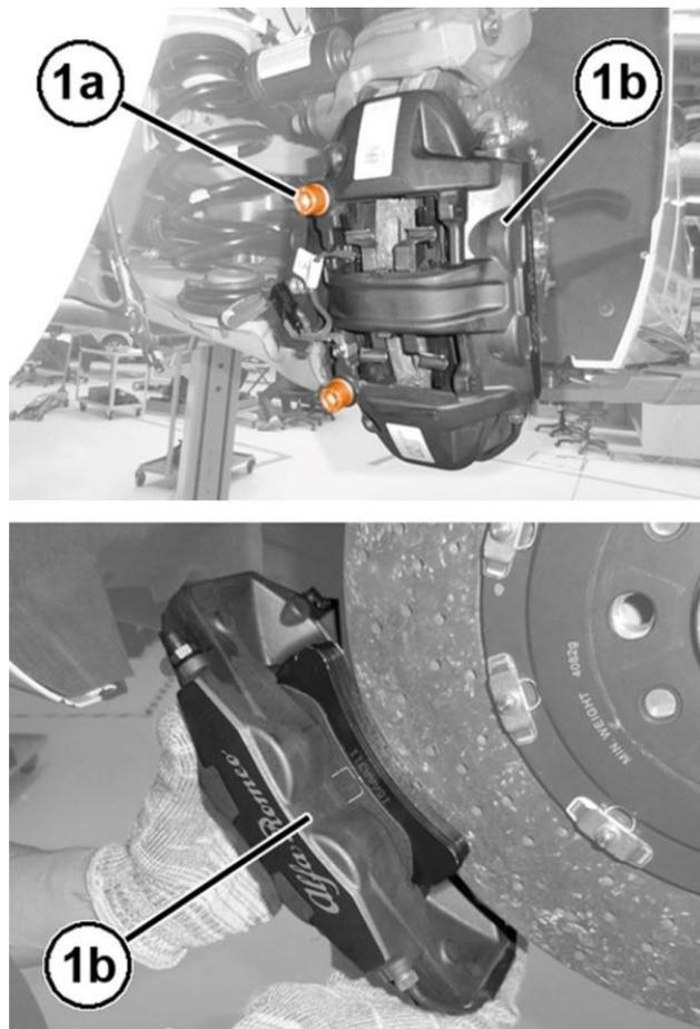
**Figure 7 – Brake Caliper**
