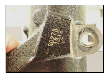
Inspect left front and right front wheel bearing housings and replace if necessary.
