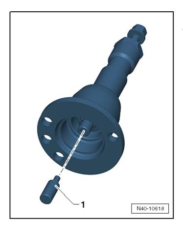
If the Drive Axle Cannot Be Pulled out of the Wheel Bearing, Then the Drive Axle Can Be Pushed out of the Wheel Bearing Using the Drive Shaft Remover -T10520A- as follows:
