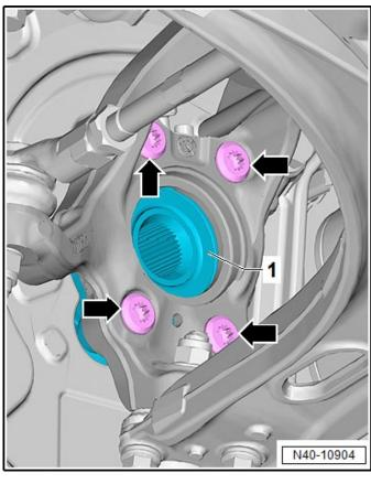
Install new wheel bearing into wheel bearing housing:
