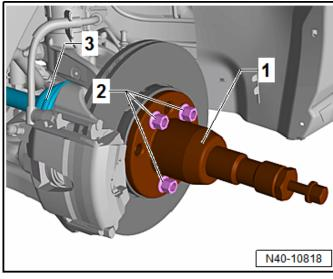
Secure the -T10520A- <1> with three wheel bolts <2> on the wheel hub, so that the drive axle <3> can be pressed out.
