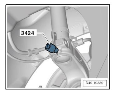
Insert -3424- into the wheel bearing housing.
