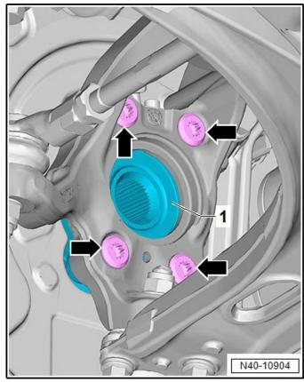
Insert -3424- into the wheel bearing housing.
