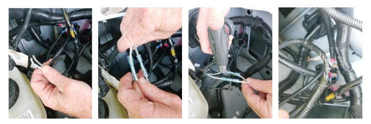
19. Zip tie fuse holders and wires together as shown below to keep secure.
