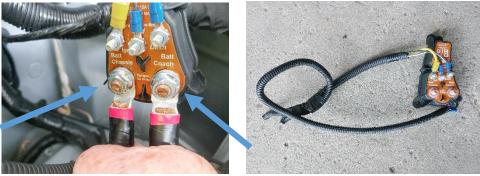
5. Remove the screws holding the BIM/BIR to the inside fender.
