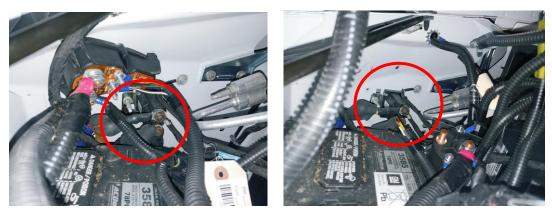
10. Start a ¼" self-tapping hex head screw at the installation mark on the fender wall. Slide Trombetta solenoid bracket into place on the self-tapping hex head screw and secure.
