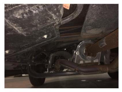
If nearby, verify the 2 gauge cable that runs from the Trombetta is supported away from the engine exhaust manifold and the rest of the exhaust, covering the area under the hood to the rear of the cab. If the 2 gauge cable is not secured away from the exhaust manifold or the rest of the exhaust, secure as indicated in the following image.
