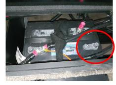
2. Disconnect battery cable from negative post of the chassis battery located under the hood.
