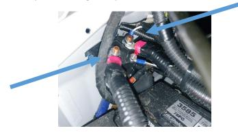
17. Locate and cut yellow ignition power wire, strip back, and connect to yellow wire w/ yellow butt connector from the fuse holder. Crimp and heat shrink using a torch or electric heat gun. Using electrical tape, tape both ends of the yellow wires.
