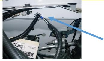
NOTE: Must use a star washer between the ring terminal and fender.
