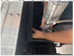
STEP 5: ENSURE THE RIVET HAS FULLY ATTACHED, THERE SHOULD BE NO GAPS BETWEEN RIVET AND THE STEEL BRACE. ONCE RIVETS ARE INSTALLED IT SHOULD LOOK SIMILAR TO THIS;
