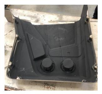
4. Using the flat blade screwdriver, remove the bonded flange and seal from the bottom of the cover.
