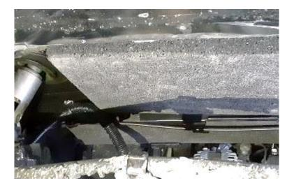
9. Using the self-drilling/tapping screws, install the 2" x 20" bracket (bracket 3 in the diagram) using the pre-drilled holes. Make sure you center the bracket correctly onto the floorboard pan frame so the screws go into the metal and not the foam. When the brackets are in proper position they will securely supports the foam insert.
