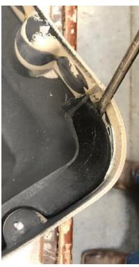
5. Insert the foam insert into the cover. Install the seal to the foam on the outer edge.
