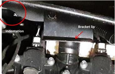
Install the 29.5" foam into the floorboard pan. The (2) brackets you just installed will secure the one side of the foam insert. Before installing the insert, make sure the angles and notch are in the right place according to the shape of the pan.
