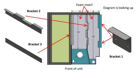
Bracket and Foam Installation Configuration
