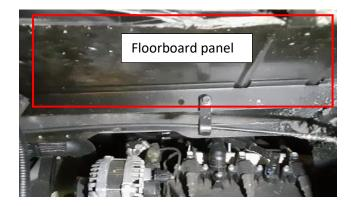
You will need to remove a cable and a line of conduit running across the floorboard panel so that you are able to install the foam insert(s). Using a screw gun and 10mm socket driver, remove the screws that are holding the cable bracket in place. You may need the 10mm open end wrench to hold the screw cap in place while removing the screw. Let both lines drop; you will re-install these in a later step. Discard the screws.
