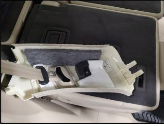
• Set the C-pillar trim down on the back of the seat as shown.
