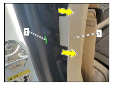
Pull the upper sill trim <1> away from the body and out of clip <2> in direction of <arrows>, ensuring that clip <2> is not bent inward.
