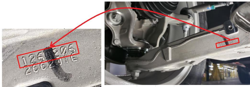
Figure 1 – Lower Control Arm Lot Number Inspection
