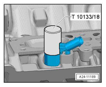
• Push the -T10133/18- over the fuel injector.
