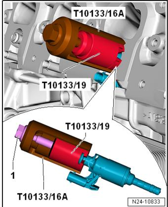
• Carefully hit the sleeve to loosen the fuel injector.
