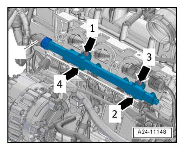
Replacing fuel rail bolts:
