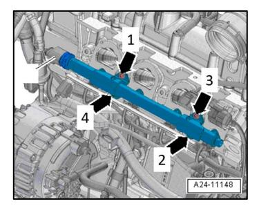
Inspect fuel rail bolts and replace fuel rail and injectors, if necessary.
