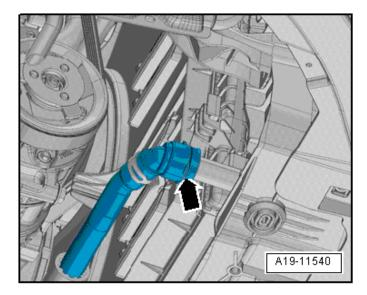
Drain engine coolant:
