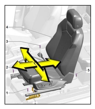
Adjust seat to highest position and perform wobble test on seat.
