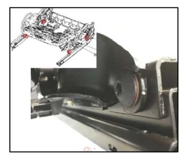
Inspect all four bolts securing the upper seat frame (seat pan) to the seat frame rails on the left front seat.
