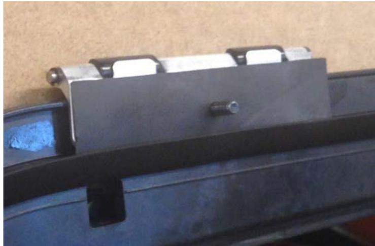
9. Install “E” clips onto the hinge pins.
