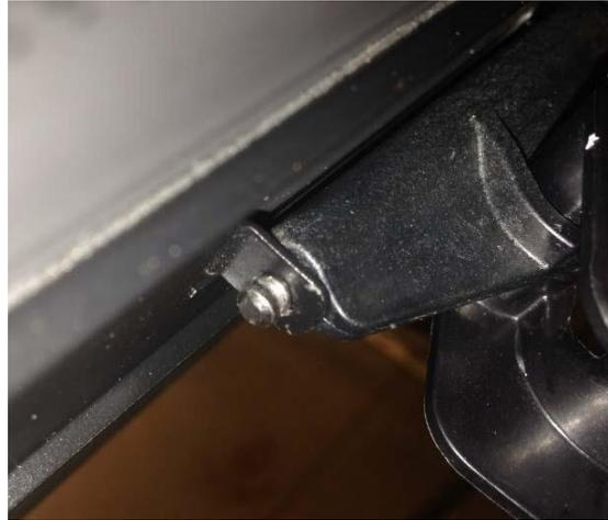
14. Install an "E" clip on the latch pin.
