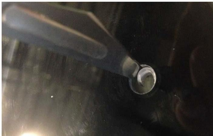
7. Install the “E” clip from the kit on one side of each new hinge pin. There should be 4 pins in total.
