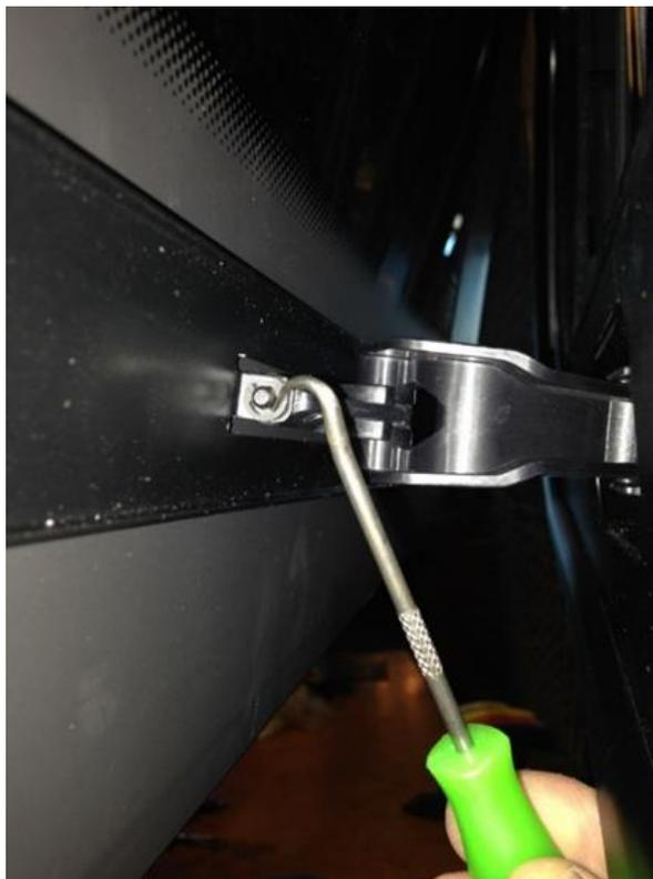
4. Remove the pin that secures the latch to the glass.
