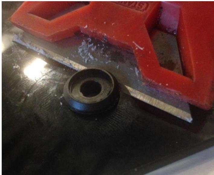
6. Remove the old glue from the mounting holes.
