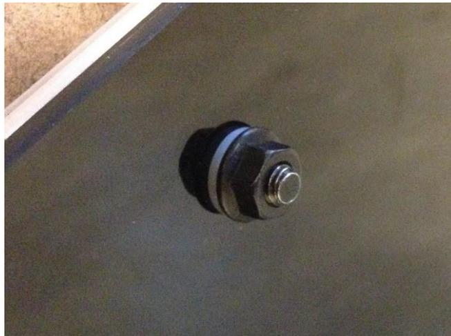
12. Install the two nut caps. Ensure the nut covers are fully seated.
