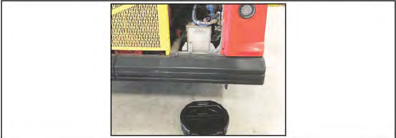
Figure 1 - Place Container to Collect Hydraulic Oil
