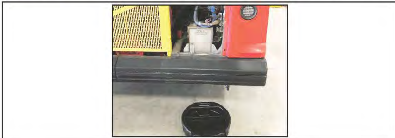
Figure 1 - Place Container to Collect Hydraulic Oil
