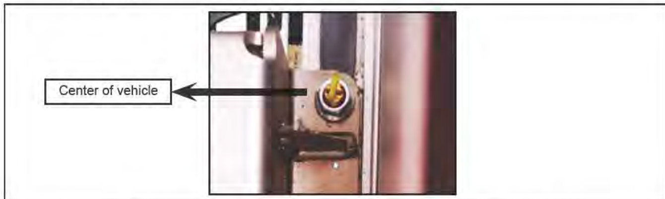
Figure 14 - The Notch of the T-Bolt Aligned Towards the Center of the Vehicle
