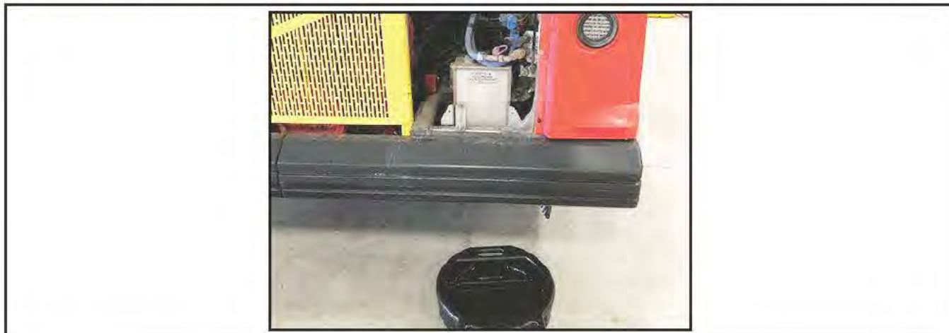
Figure 1 - Place Container to Collect Hydraulic Oil
