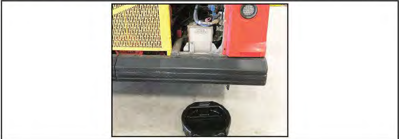
Figure 1 - Place Container to Collect Hydraulic Oil
