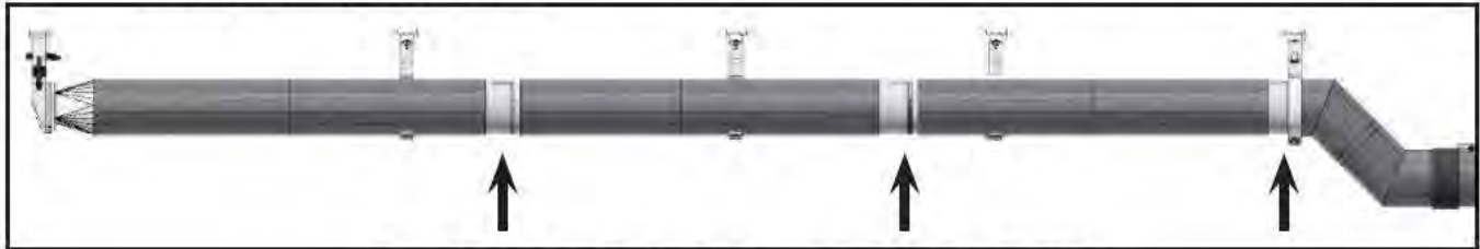
Figure 8 - Remove the Insulation and the Aluminum Foil Tape
