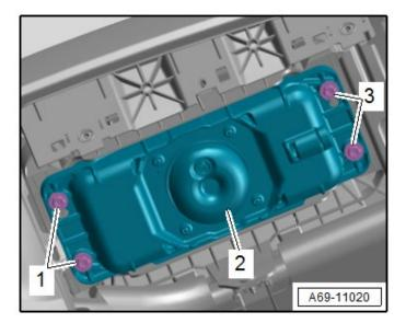
Support the Front Passenger Airbag Unit <2> to prevent it from falling out.
