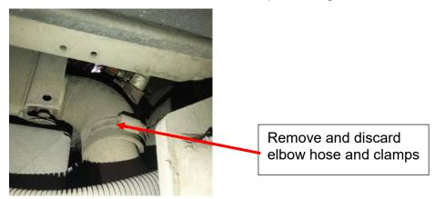
Install the new elbow hose, MCI P/N: 06-08-2261, using new clamps, MCI P/N: 19-04-0520. Torque the clamps to 105 In-Lb.
