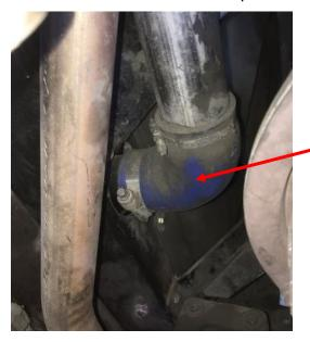
Remove and discard elbow hose and clamps
