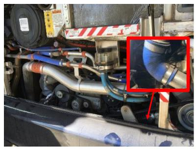
Remove and discard the coolant hose elbow and the two hose clamps.
