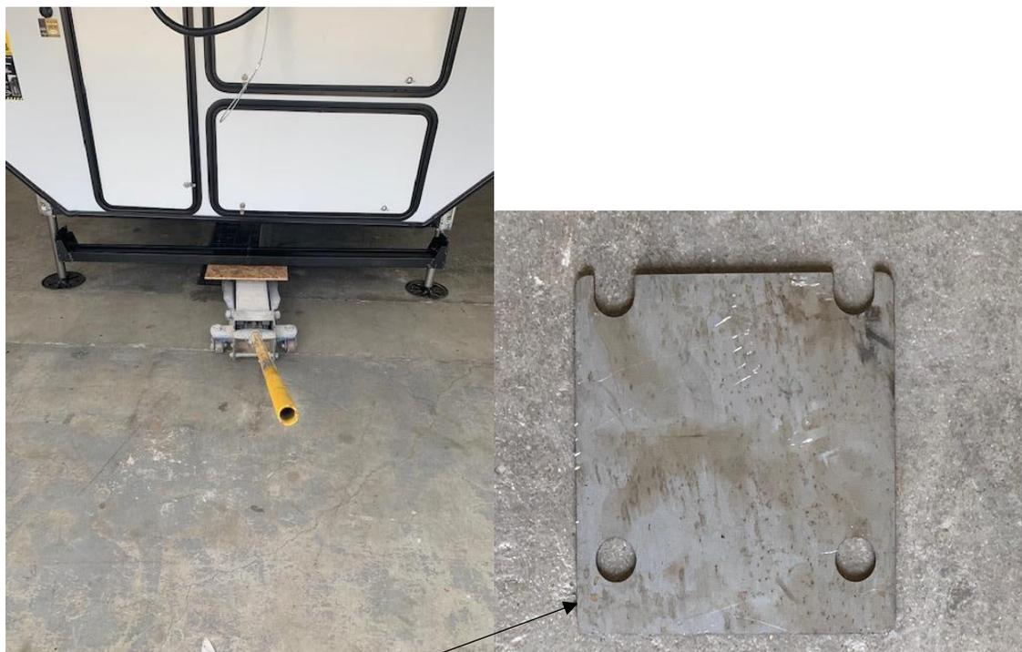
5. Use the provided shims that are 1/8" & 1/4" thick to ensure that the bracket has no more than a 1/2" gap to be closed up when tightening bolts. (Some brackets may not require any shims & will have less than 1/2" gap once in place)
