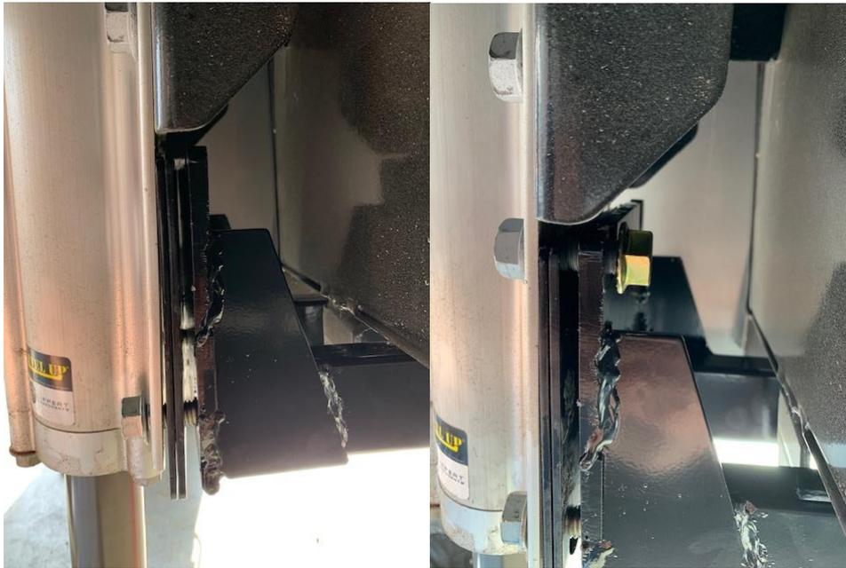
17. Once you have all the bolts on both sides of the bracket snug all bolts down until tightened.
