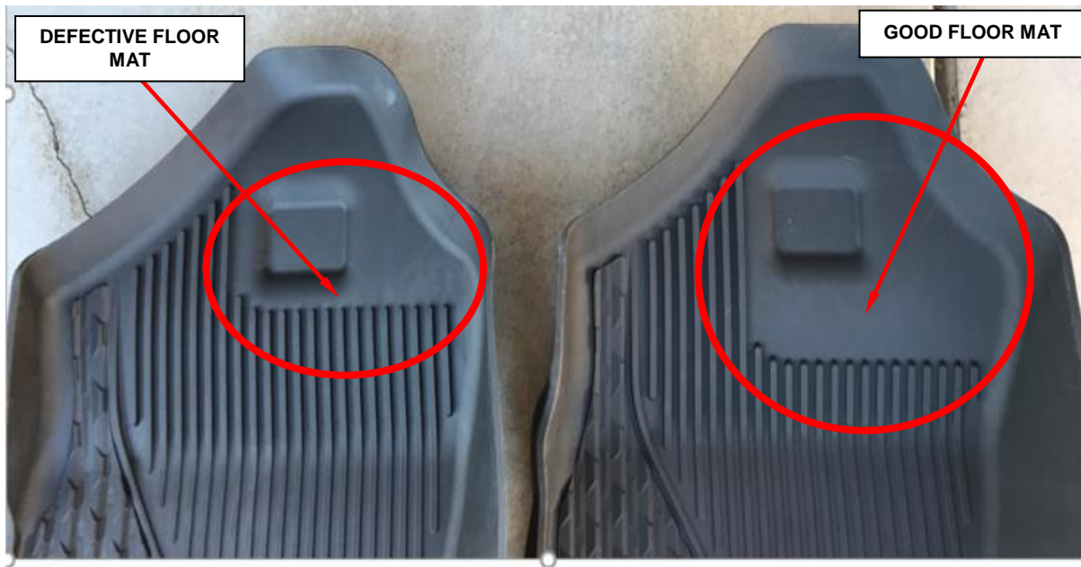
Figure 1 – All-Weather Drivers Side Floor Mat
