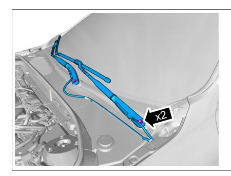
Caution! Hold the marked component in position to keep it from moving.
