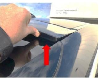
3. While pressing upwards using a thumb and moderate force, measure the gap between the glass and the bottom of the rear spoiler (arrow) again.
