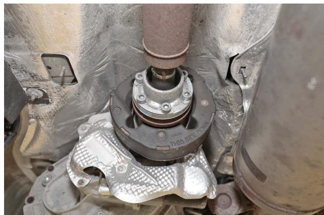
Figure 30 – Propeller Shaft at Transfer Case
