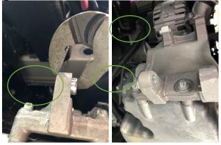
Place the top bolt into the mounting bracket just far enough to hang the black spacer flush on the end. Move the alternator into place and slide bolt through and hand start threading. Make sure the spacer stays in place. Place bolt through negative cable and spacer on the bottom mount in the same orientation. Thread both bolts on equally to the point where they just begin to tighten. Then rotate a quarter turn back and forth between the two until tight. Torque to 34.5ft/lbs
