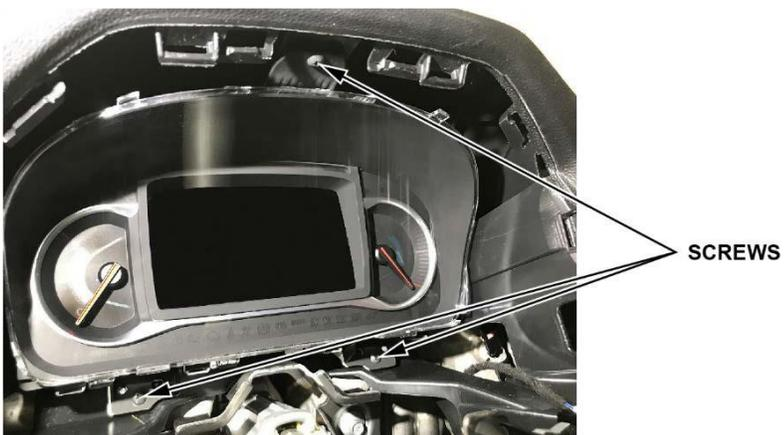
8. Turn the gauge control module to access the rear connectors, being careful not to stretch the wiring harness. Disconnect the red and green FAKRA connectors, then disconnect the remaining connectors, and remove the gauge control module from the vehicle.
