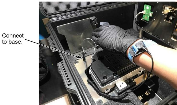
3. Connect the grey connector to the gauge control module.
