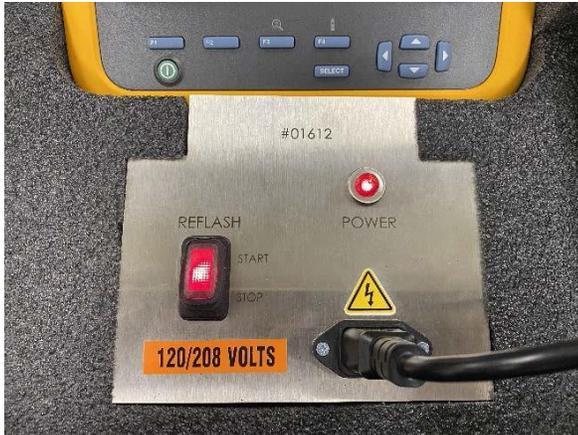
9. Check the reflash status through the inspection mirror below the gauge control module. The reflash will take about **7 to 10 minutes** to complete.
