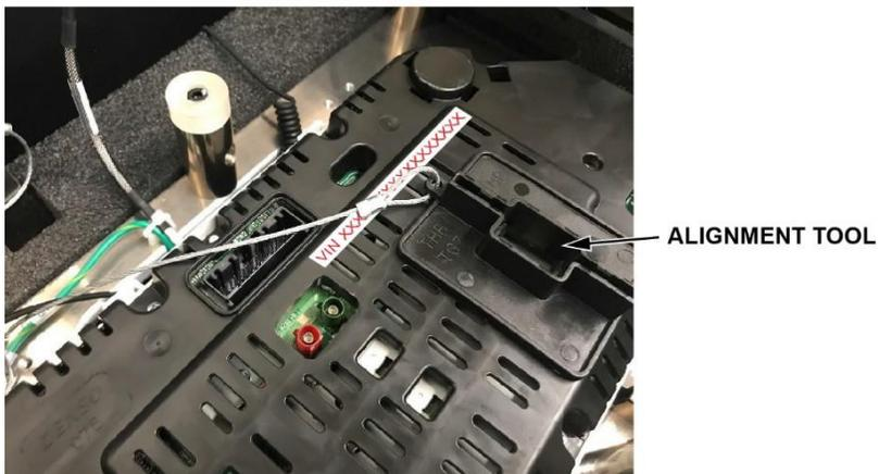
4. Connect the grey connector into the gauge control module.
