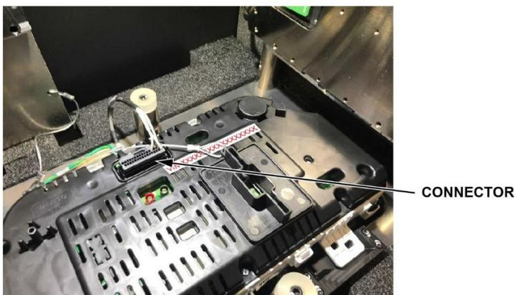
5. Insert the SMART reflash card into the alignment tool, making sure the connectors make good contact.
