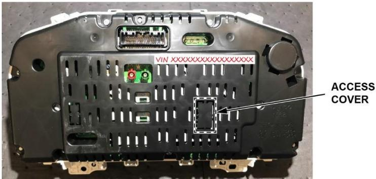
NOTE: Some gauge control modules have a connector on the circuit board and some do not.
