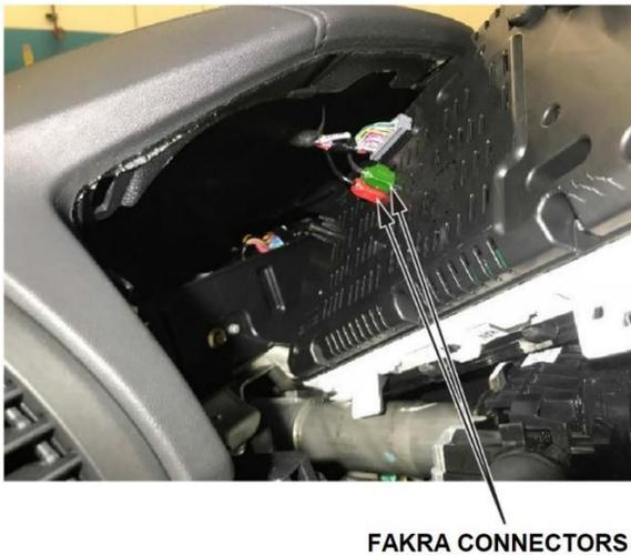
NOTE: Make sure the harness is straight and not wrapped or tangled with other wires.
