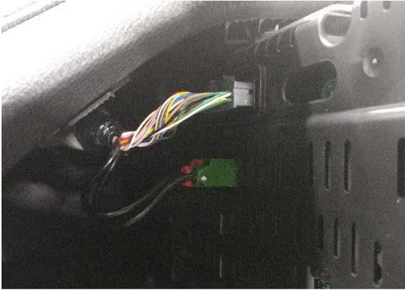
9. Write the VIN on a piece of tape and attach it to the back of the gauge control module.
