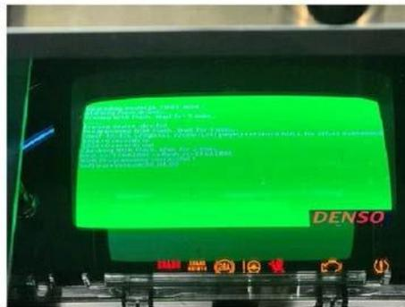
*If the reflash fails, set the REFLASH toggle switch to STOP and remove the SMART reflash card. Then, start REPAIR PROCEDURE B again from step 5.*
