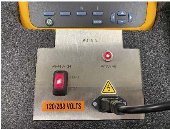
7. Check the reflash status using the inspection mirror under the gauge control module. The update will take about **7 to 10 minutes** to complete. The screen will turn green once the reflash is complete.
