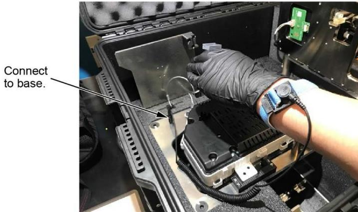
3. Set the alignment tool in the access hole in the gauge control module.
