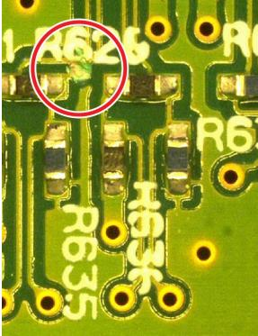
We've concluded this damage happened when either removing the access cover from the back of the module or when lowering the pogo head onto the circuit board with the Z-axis control knob. You can easily damage this printed circuit board when doing either of those actions, so you need to be extra careful.
