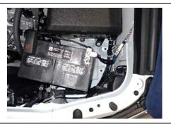
b. Reposition the battery as far inboard as possible.
