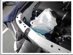
b. Reposition the reservoir as far inboard as possible.
