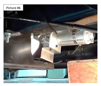
7. Install the original lock washer and nut onto the pump bolt securing the pump to the bracket.
