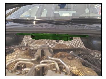
• Install new engine compartment seal retaining plate.
