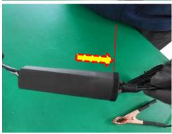
6. Using a heat gun, carefully shrink the tubing over the connector.
