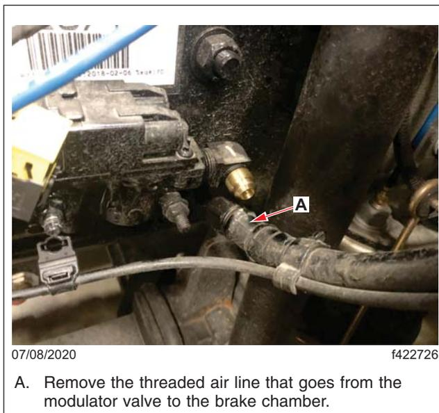
**Fig. 7, Removing the Threaded Air Line**
