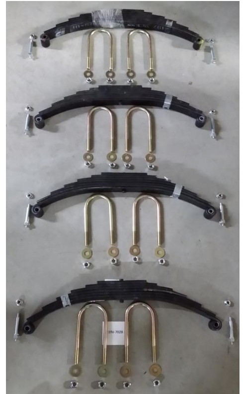
STEEL LEAF SPRINGS 20V-385B Required based upon inspection results
