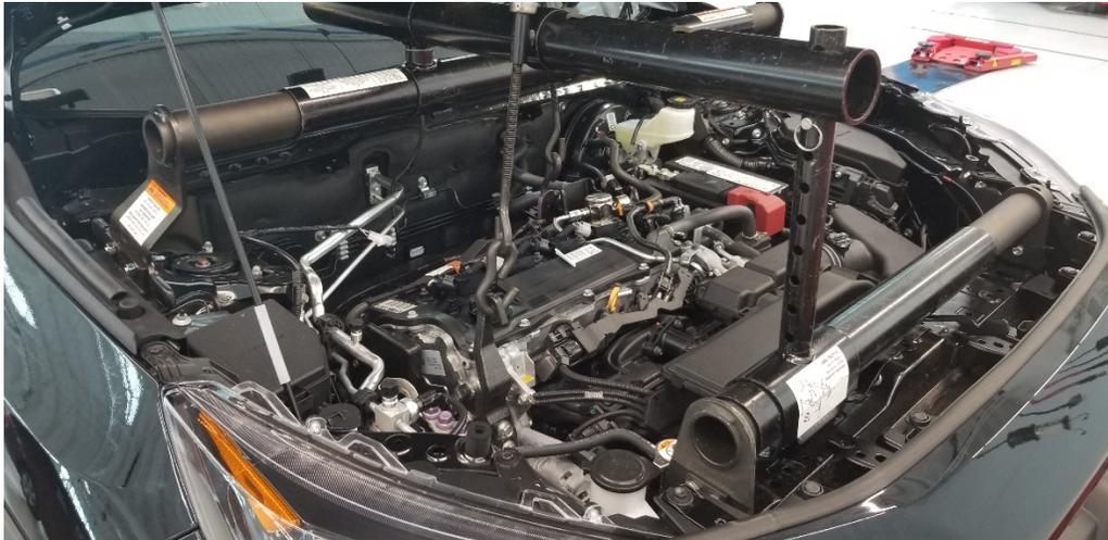
Picture of final Engine Support Bar assembly for reference
