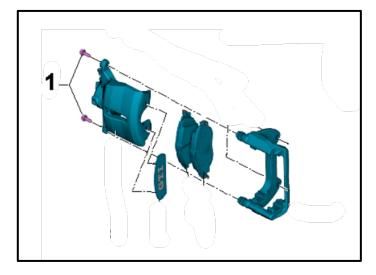
Replace left front and right front brake caliper bolts <1>.
