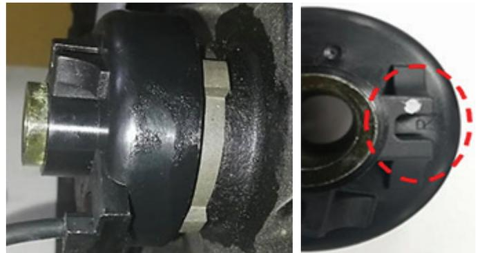
Reassemble the front wheel, pay attention to the front wheel speed sensor, the front shock mount is inserted into the U-shaped slot at the white dot mark and/or the R engraved in card.
