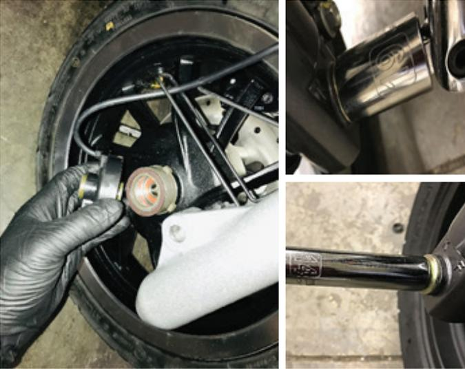
Remove the axle screw to drop front wheel. Separate ABS cover from sensor ring. (14mm bolt head and 19mm nut)
