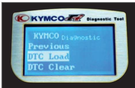
Once back on the first page, press the right (down) button to scroll down to **DTC inspection**. Press the ENTER button on the **DTC Inspect** to move to next screen.
