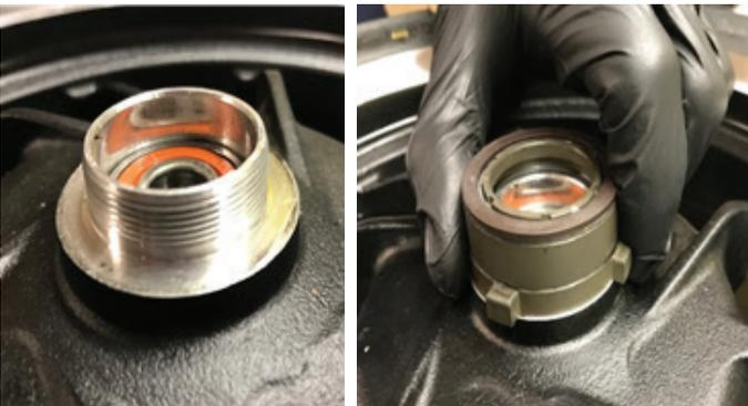
Remove the damaged speed sensor magnetic ring. Install the new magnetic ring from the recall kit. Screw-on the sensor snug-tight by hand.
