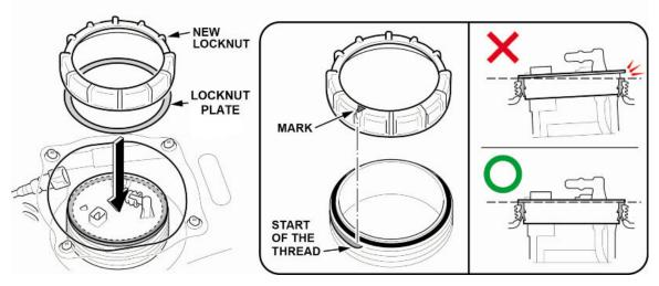
11.2. Tighten the fuel tank unit locknut to the specified torque using the fuel sender wrench.
