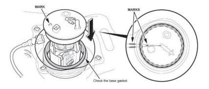
11. Tighten the fuel tank unit locknut.
