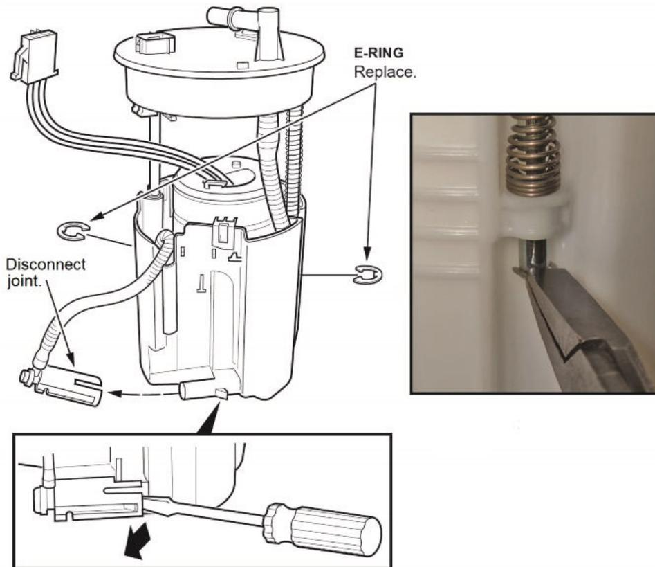
8.5. Disconnect the joint at the bottom of the reservoir.
