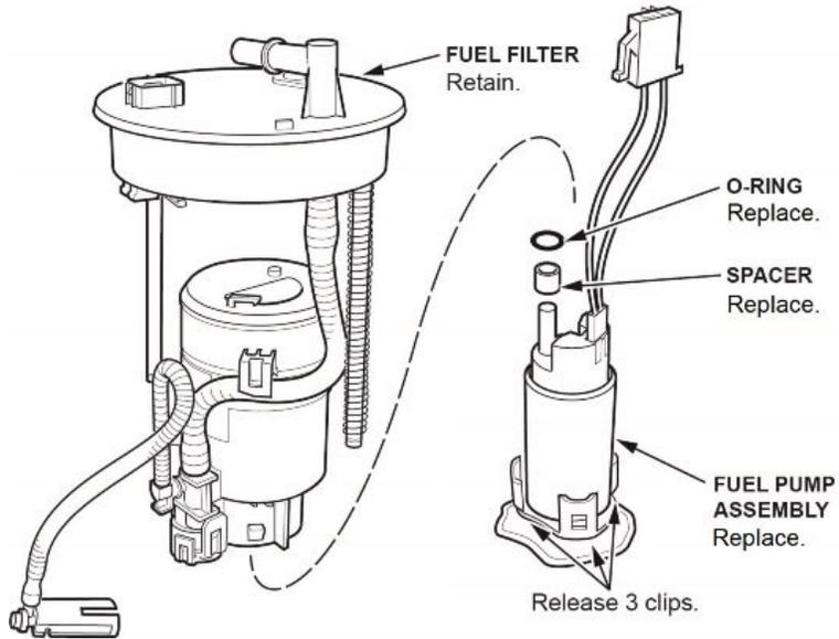
9. Assemble the fuel tank unit.
