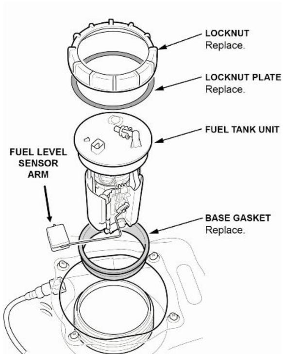
8. Disassemble the fuel tank unit.
