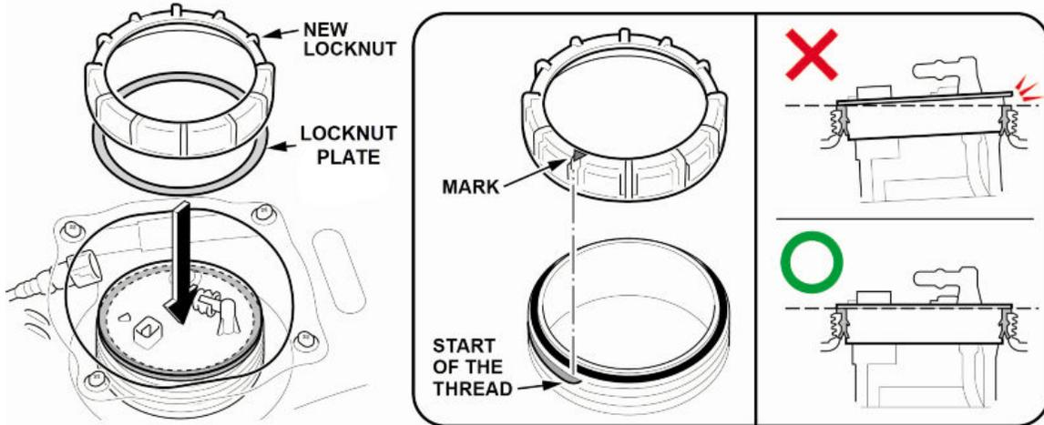
11.2. Tighten the fuel tank unit locknut to the specified torque using the fuel sender wrench.
