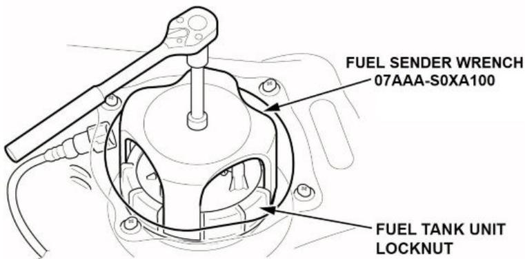
7. Remove the fuel tank unit locknut, and remove the fuel tank unit.
