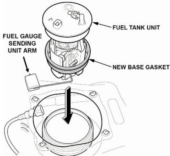
10.2. Line up the marks on the fuel tank and fuel tank unit, then insert the fuel tank unit into the fuel tank.
