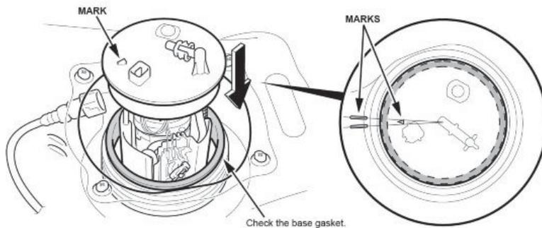
11. Tighten the fuel tank unit locknut.
