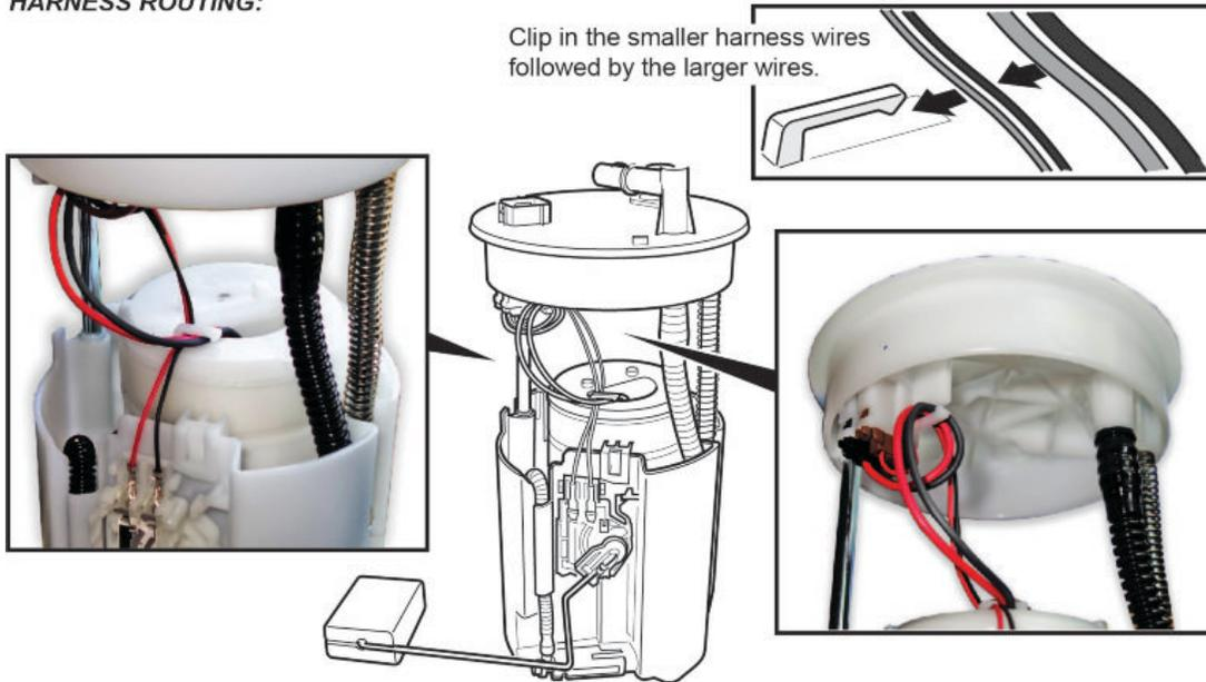
9.7. While compressing the fuel tank unit, make sure the movement is smooth and the fuel tube and wiring harness do not pinch or bind.
