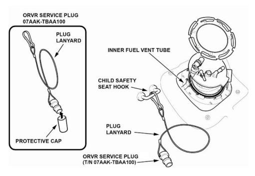
11.2. Disconnect the inner fuel vent tube from the fuel tank unit, and hold it. Do not allow the inner fuel vent tube to drop into the fuel tank.
