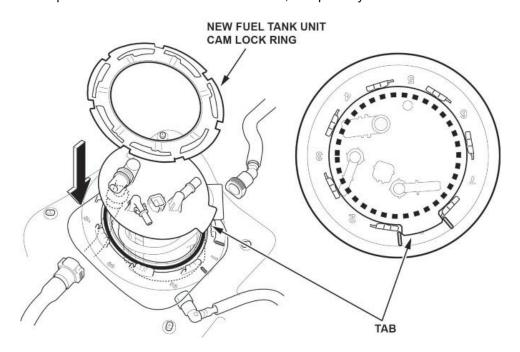
15. Connect the fuel vent tube and fuel tank vapor recirculation tube by slightly turning the fuel tank unit counterclockwise.
