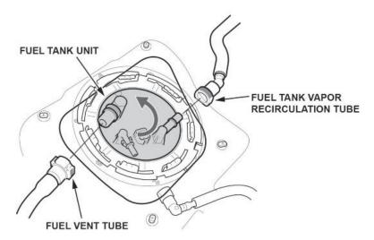
16. Tighten the fuel tank unit cam lock ring.
