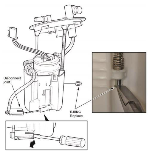
12.5. Disconnect the joint at the bottom of the reservoir.
