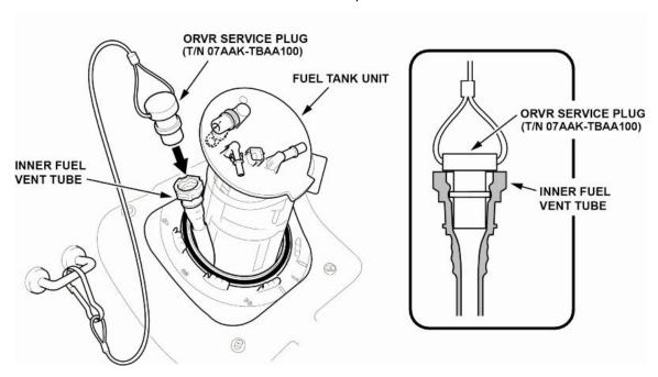
11.3. Install the ORVR service plug to the inner fuel vent tube. Make sure the ORVR service plug is fully seated by holding the inner fuel vent tube, and gently pulling on the plug's lanyard.
