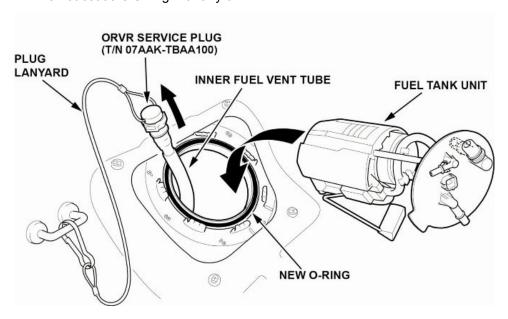
14.2. Grab the plug lanyard, and pull the inner fuel vent tube up until it is close to the fuel tank opening.
