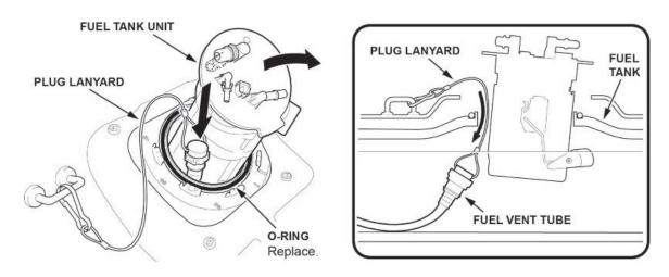
11.5. Remove the fuel tank unit with the O-ring.
