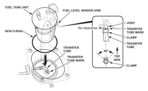
10.2. Align the marks on the fuel tank and fuel tank unit, then insert the fuel tank unit into the fuel tank.
