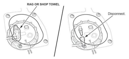
6. Unlock the fuel tank unit locknut using the fuel sender wrench (T/N 070AA-T0AA100).
