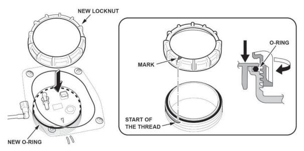
12. Tighten the fuel tank unit locknut to the specified torque using the fuel sender wrench.
