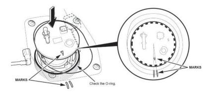
11. Tighten the fuel tank unit locknut.
