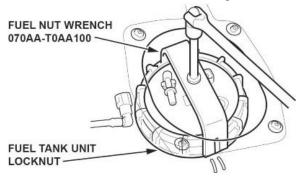
7. Remove the fuel tank unit locknut, and lift it up just enough to disconnect the transfer tube. Then, remove the fuel tank unit.
