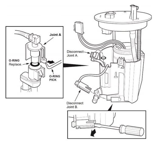
8.6. Disconnect Joint B from the bottom of the reservoir.
