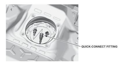
Connect the fuel tank unit connector.
