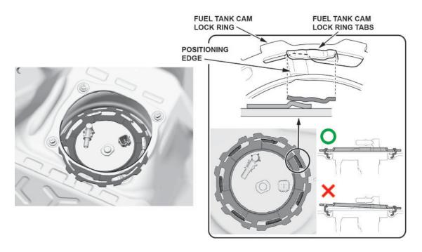
11.2. Turn the fuel tank unit cam lock ring clockwise using the fuel sender wrench.
