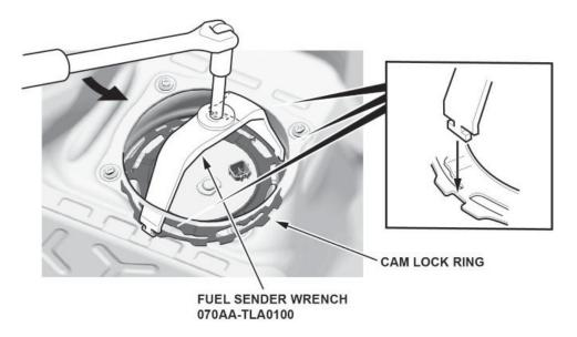
6.2. Turn the fuel tank unit cam lock ring counterclockwise.
