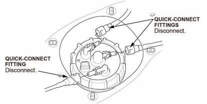
17. Loosen the fuel tank unit locknut using the Fuel Sender Wrench (T/N 07AAA-S0XA100).
