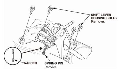
13.2 Remove the shift lever housing bolts.
