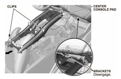
9. Remove the center console rear trim, and disconnect the connector.
