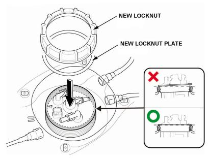
22.2. Tighten the fuel tank unit locknut to the specified torque using the fuel sender wrench.
