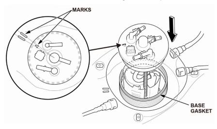
22. Tighten the fuel tank unit locknut.
