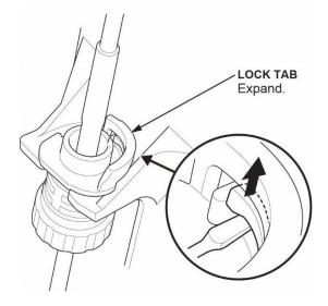
14.5 Rotate the socket holder retainer counterclockwise until it stops, then remove the shift cable.
