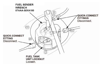
18. Remove the fuel tank unit locknut, then remove the fuel tank unit.
