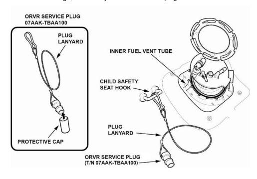
12.2. Disconnect the inner fuel vent tube from the fuel tank unit, and hold it. Do not allow the inner fuel vent tube to drop into the fuel tank.
