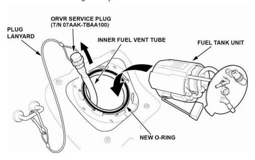
15.2. Grab the plug lanyard, and pull the inner fuel vent tube up until it is close to the fuel tank opening.
