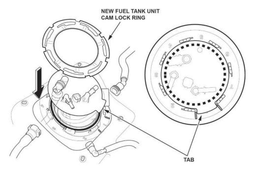
16. Connect the fuel vent tube and fuel tank vapor recirculation tube by slightly turning the fuel tank unit counterclockwise.
