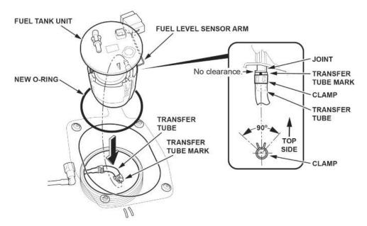
12.2. Align the marks on the fuel tank and fuel tank unit, then insert the fuel tank unit into the fuel tank.
