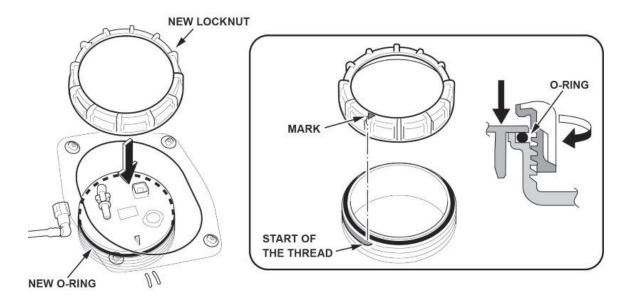
14. Tighten the fuel tank unit locknut to the specified torque using the fuel sender wrench.
