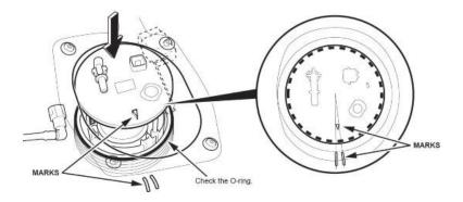
13. Tighten the fuel tank unit locknut.
